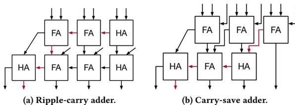
Figure 4: Examples of two types of adders.
