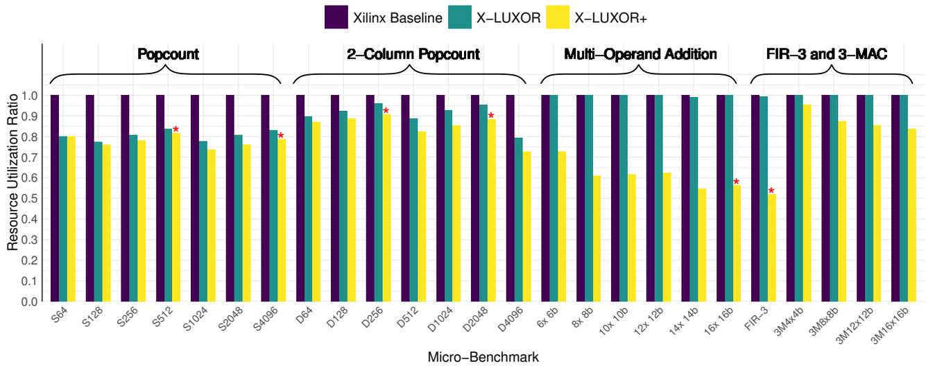
**Figure 11: Resource reduction on Xilinx UltraScale+, X-LUXOR, and X-LUXOR+ architectures for various micro-benchmarks. The \* indicates that the proposed solution required one less logic stage in the compression tree.**
