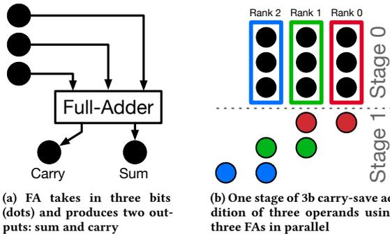
Figure 1:  $(3:2)$  parallel counter, also known as a full-adder.
