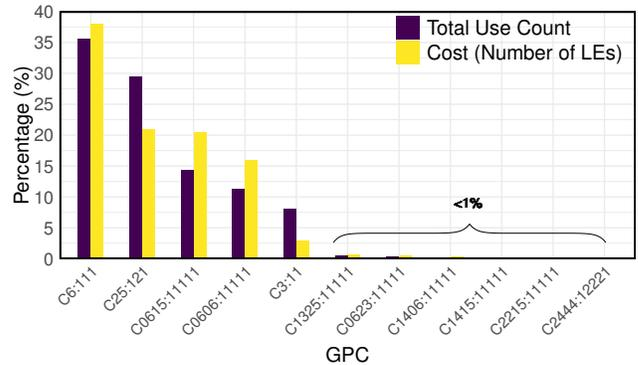
**Figure 6: Total percentage count and cost of each GPC/compressor found in optimal solutions of compressor trees across 50+ Micro-Benchmarks from a variety of fields. The GPC/compressor list is according to [22]**
