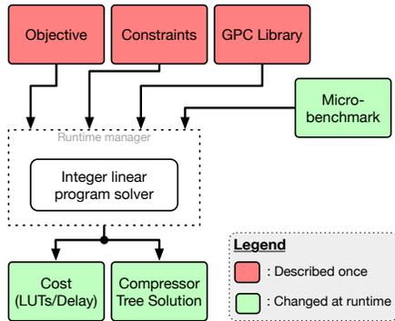
Figure 10: Flowchart of ILP-based compressor tree synthesis
