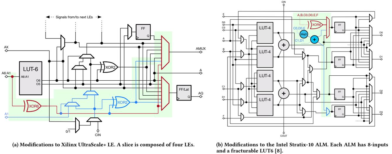
**Figure 5: Basic logic element (LE) for Xilinx and Intel FPGA architectures. LUXOR modifications are highlighted in red, while vendor-specific LUXOR+ modifications are colored blue. Some signals are omitted for simplicity.**
