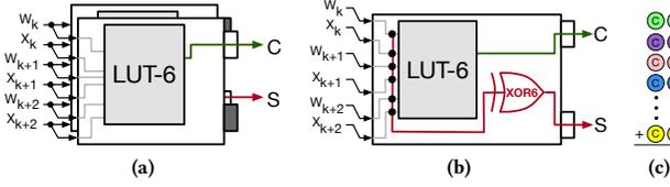
**Figure 7: BNN implementation on Xilinx FPGAs: primary multiply and compressors of (a) XnorPopcount with 2 LEs, (b) XnorPopcount with 1 LUXOR LE. (c) Final two-column popcount to accumulate the partial sums (S), and carries (C)**
