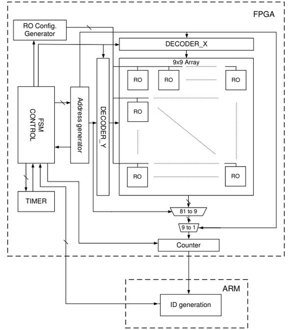
Fig. 1. Block diagram of chip ID generator.
