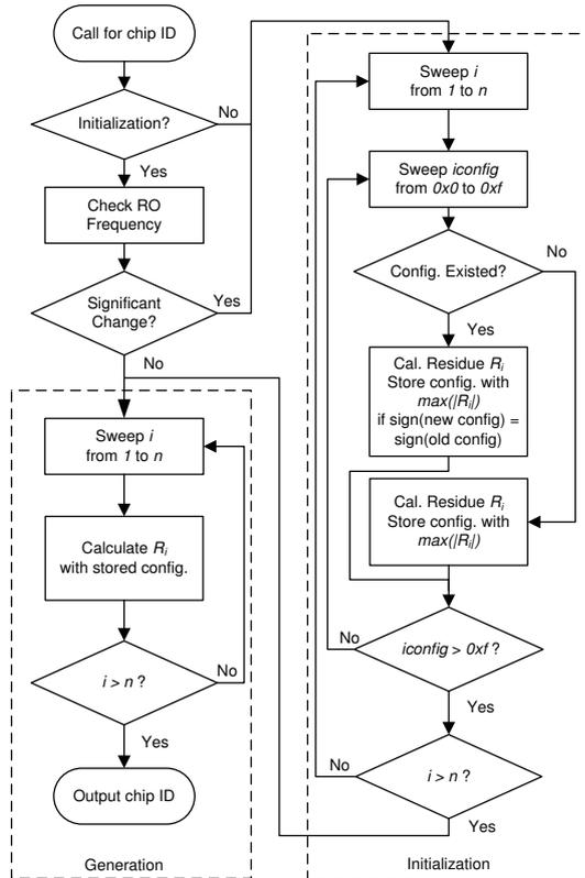
Fig. 4. Flowchart showing chip ID generation process.
