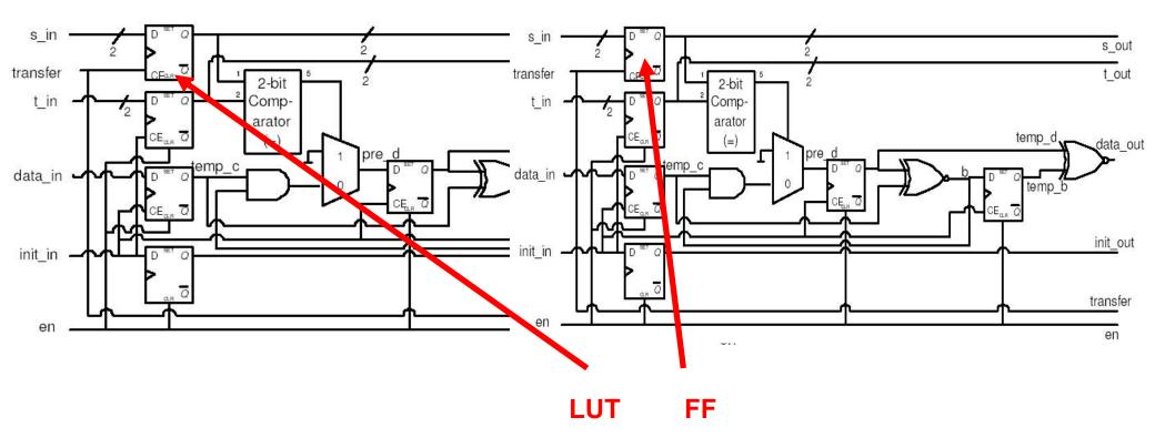
Merge two cells so that FFs are connected as in the slice (8 LUTs, 4 RAMs, 12 FFs) = 6 slices (2 cells)
