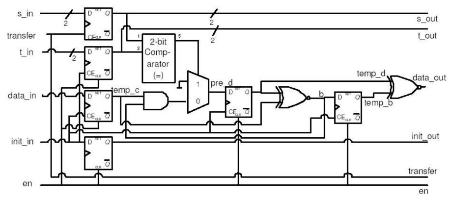
4 LUTs and 8 FFs = 4 slices Guccione's cell uses 3 slices by writing string in bitstream
