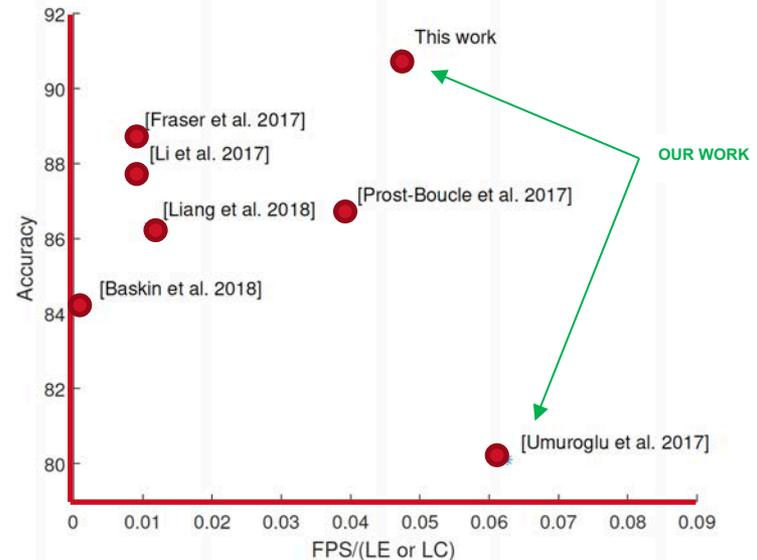
Ours is the most accurate and fastest reported FPGA-based CNN inference implementation CIFAR10: 90.9% acc, 122K fps (TRETS'19)
