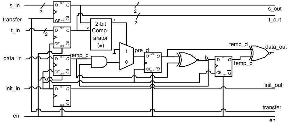
Figure 1.2. The Smith-Waterman processing element (PE). Boxes represent D-type flip-flops.
