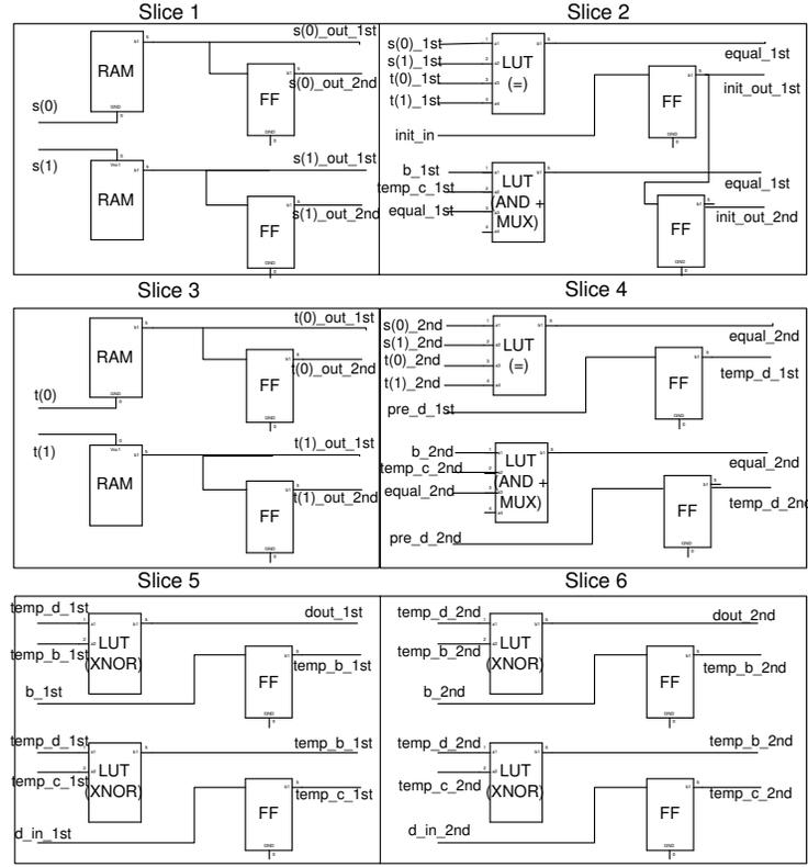
Figure 1.3. Two processing elements mapped to 6 Virtex slices.
