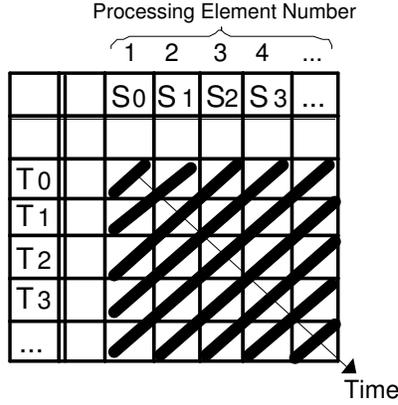
Figure 1.1. Data dependencies in the alignment table. Thick lines show entries which can be computed in parallel and the time axis is arranged diagonally.
