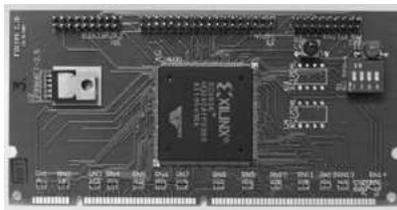
**Fig. 6.** Photograph of the Pilchard board.
