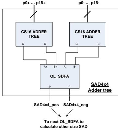
Fig. 6. 16-operand sign-digit adder tree for 4x4 SAD.
