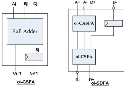
Fig. 2. On-line Carry save and signed-digit adders
