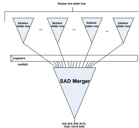
Fig. 4. Signed-digit adder tree that generates 41 SADs
