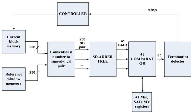
Fig. 8. SD-adder tree that generate 41 SADs
