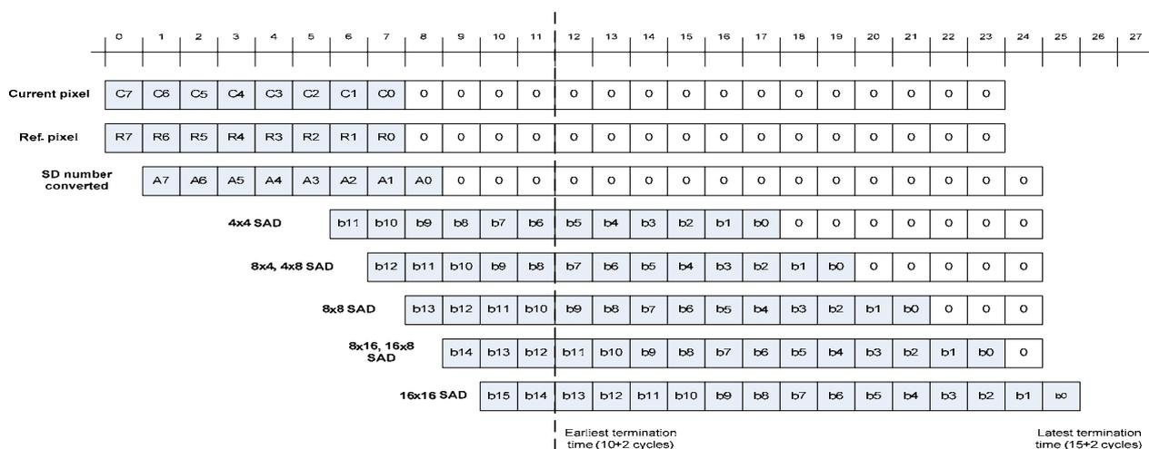
Fig. 11. Timeline for whole motion vector computation process
