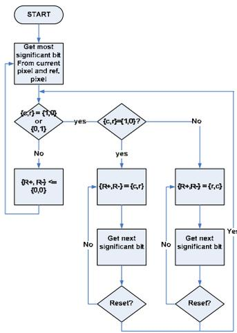
Fig. 9. Flow chart of conventional number to signed-digit conversion
