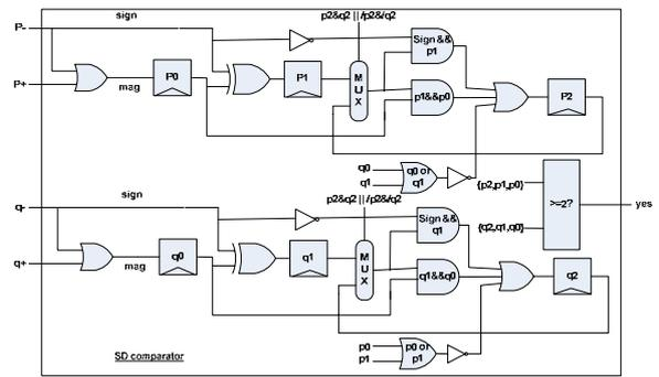
Fig. 10. Architecture of on-line comparator
