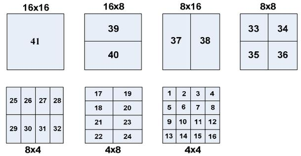
Fig. 1. Supported block sizes in H.264/AVC
