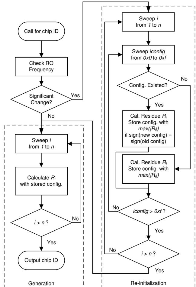
Fig. 12. Flowchart showing chip ID generation process.
