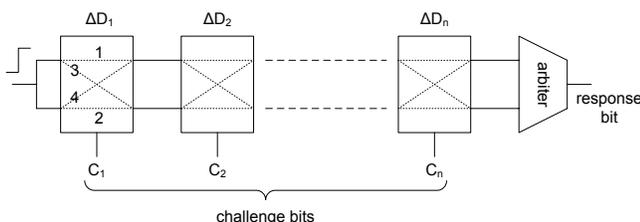
Fig. 1. Arbiter-based PUF.
