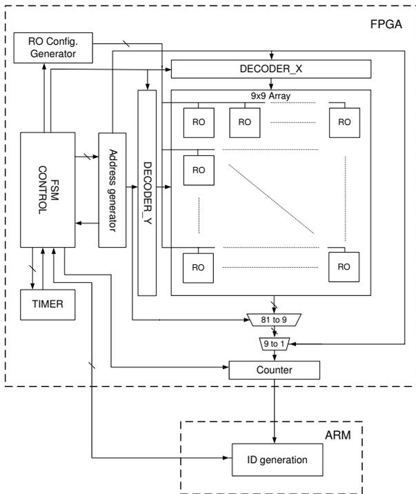
Fig. 4. Block diagram of chip ID generator architecture.
