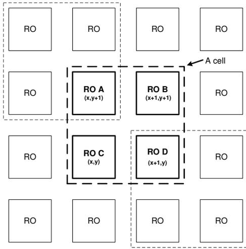
(a) Block diagram of a cell.
