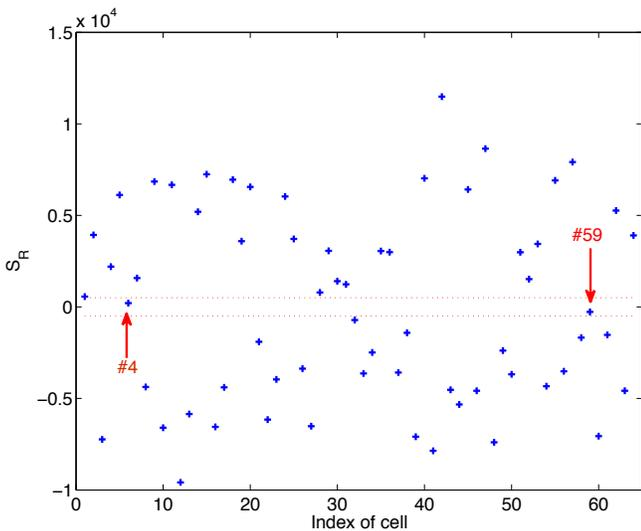
Fig. 8.  $S_R$  for all cells, cell #4 and #59 are marginal, as their  $S_R$  values fall between  $\pm 500$ .
