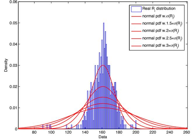
Fig. 18. A Histogram of  $R_i$  and Gaussian pdf plots with tunable standard deviation.
