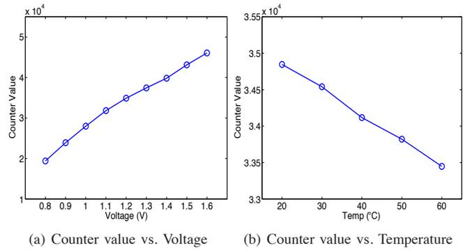
Fig. 11. Counter value vs. Voltage/Temperature
