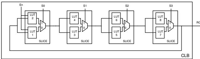
Fig. 5. Circuit for the configurable RO.
