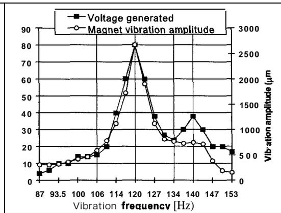
Figure 8. Voltage output and the vibration amplitude versus input frequency of an cantilever structure.
