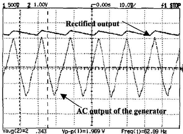
Figure 9. AC Voltage output of the generator (input vibration at 64Hz, 100μm amplitude) and DC output after rectifying the AC signal.
