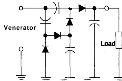
Figure 10. A quadrupler voltage rectifier to convert the AC voltage into DC output.
