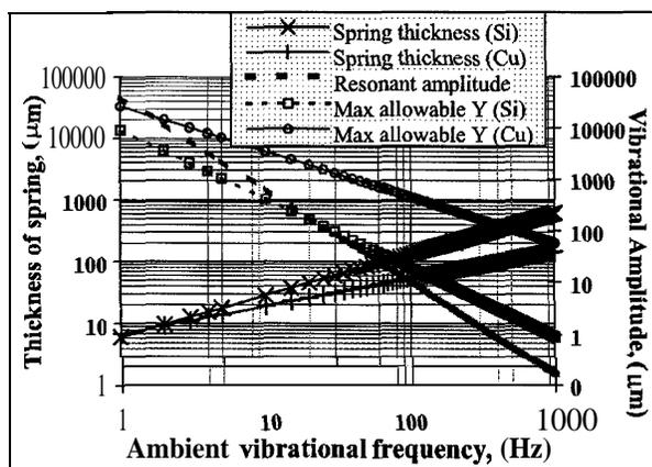
**Figure 3.** Analysis of spring thickness requirement and Maximum allowable deflection as functions of ambient Vibrational frequency.
