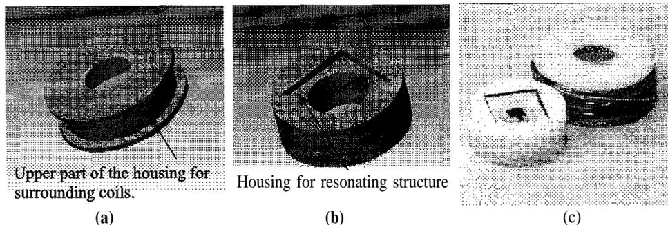
**Figure 5.** (a) Upper (outer) part for the coil. (b) Inner part for spring structure. (c) Picture of a generator. Part (a) is hollow for part (b) to fit inside it.
