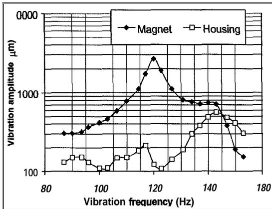
Figure 7. Vibration amplitude of the housing on top of the vibration drum.
