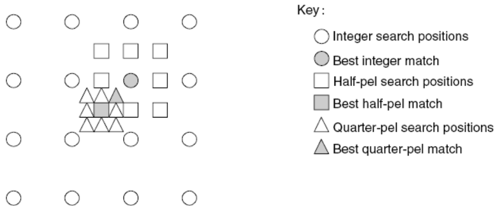
Figure 2.6: Integer, half-pixel and quarter-pixel motion estimation search positions (pel stands for pixel)
