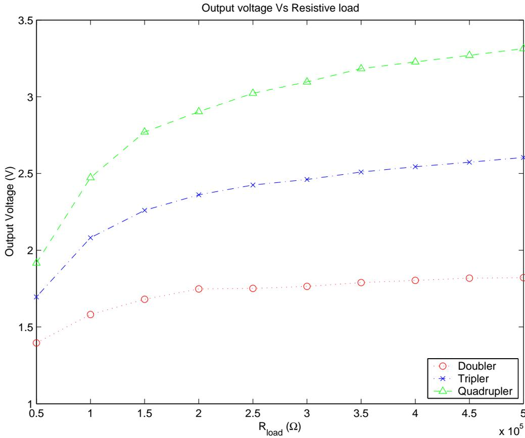
Figure 3.5: The output characteristics for voltage doubler, tripler and quadrupler with different loading (simulated by PSpice, OrCAD)
