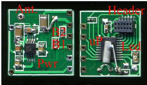
Figure 6.2: Photograph of ring board (top view)
