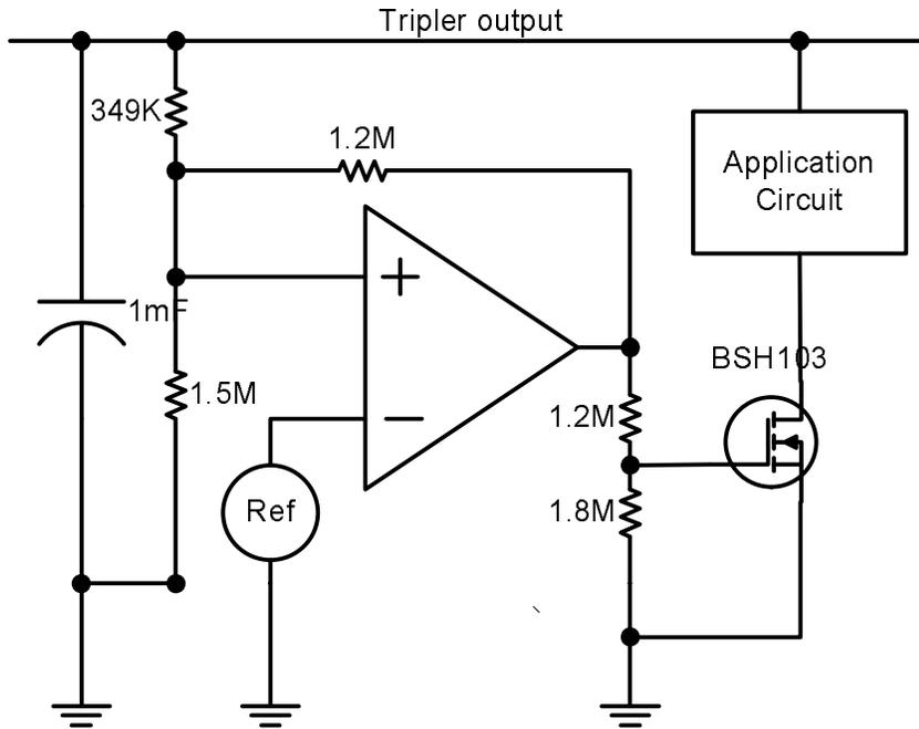
Figure 4.4: Schematic of startup module
