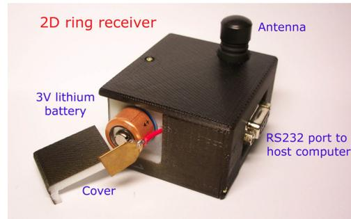
Figure 6.16: Photograph of 2D ring receiver
