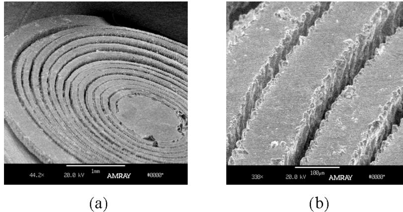
Figure 3.2: SEM pictures of: (a) a laser-micromachined copper spring with diameter of 5 mm, (b) close-up of the copper spring; width of spring is  $\sim 100 \mu m$ . Photo courtesy of Johnny M. H. Lee.
