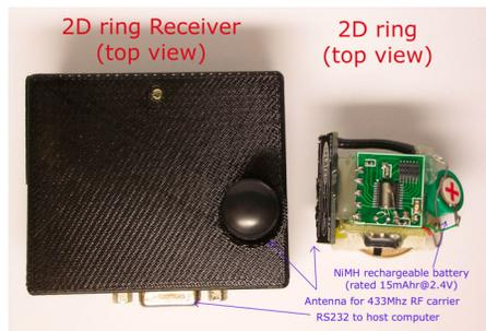
Figure 6.17: Photograph of 2D ring demo kit (top view)
