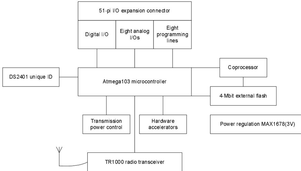
Figure 2.6: Block diagram of MICA node [14]
