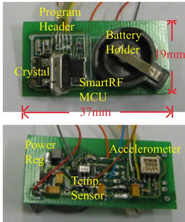
Figure 5.4: Photograph of prototype 3
