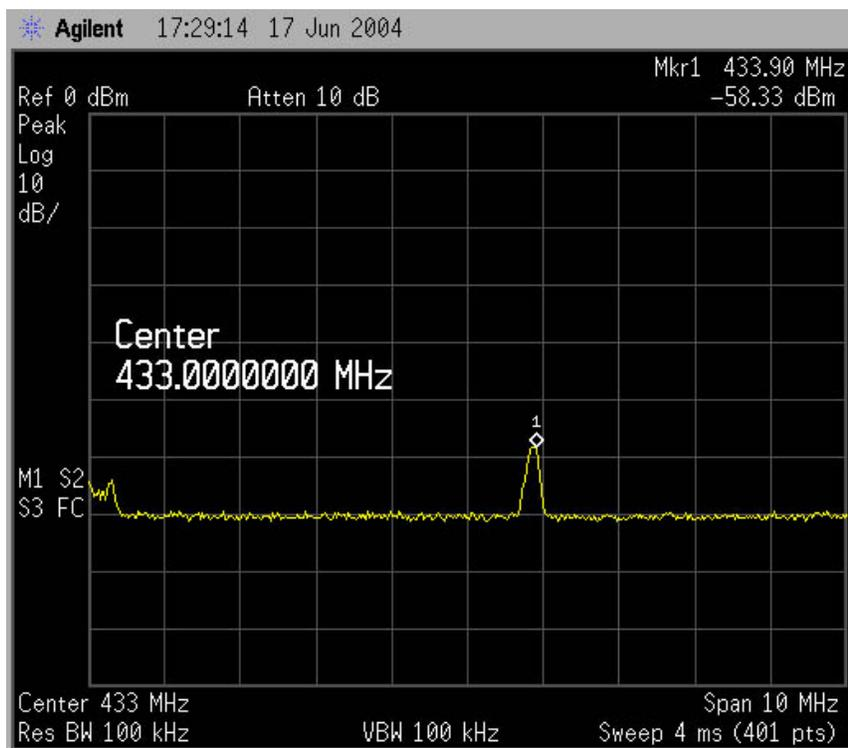
Figure 6.14: Transmission power of the 2D ring at 3 *m*
