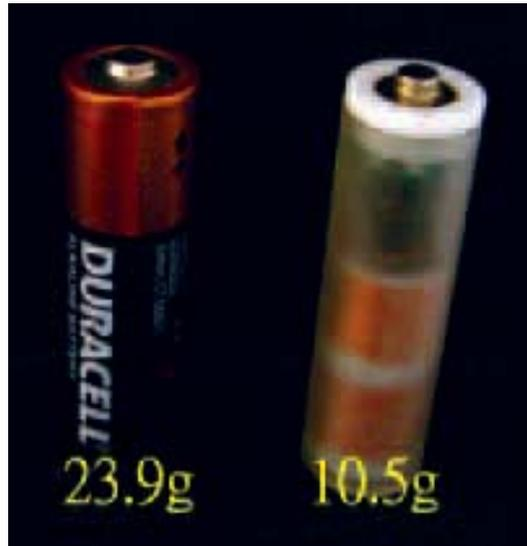
Figure 3.10: MPG (left) weighs less than the normal AA-size battery (right). Photo courtesy of Johnny M. H. Lee
