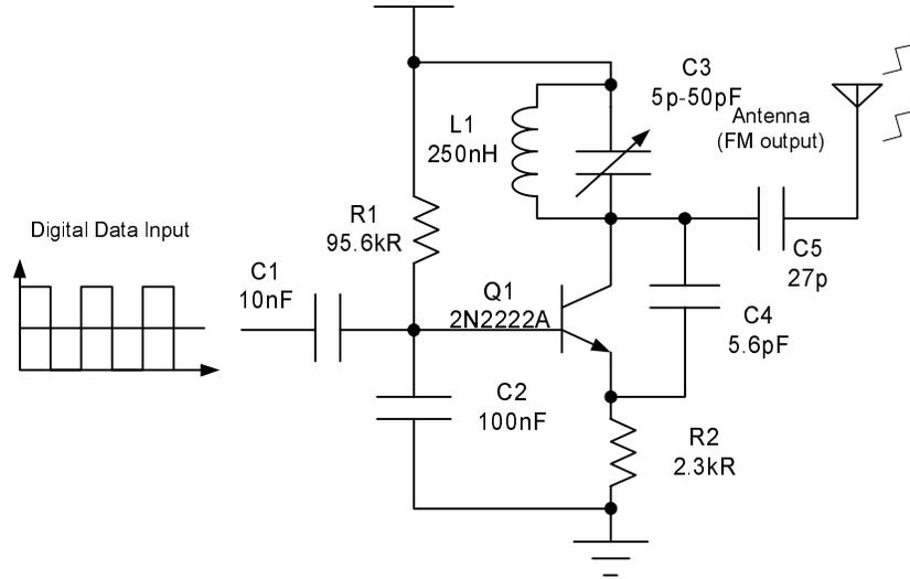
Figure 4.9: Schematic of LC-based radio frequency transmitter
