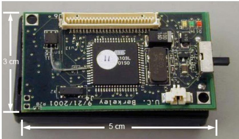
Figure 2.7: Photograph of MICA node [40]
