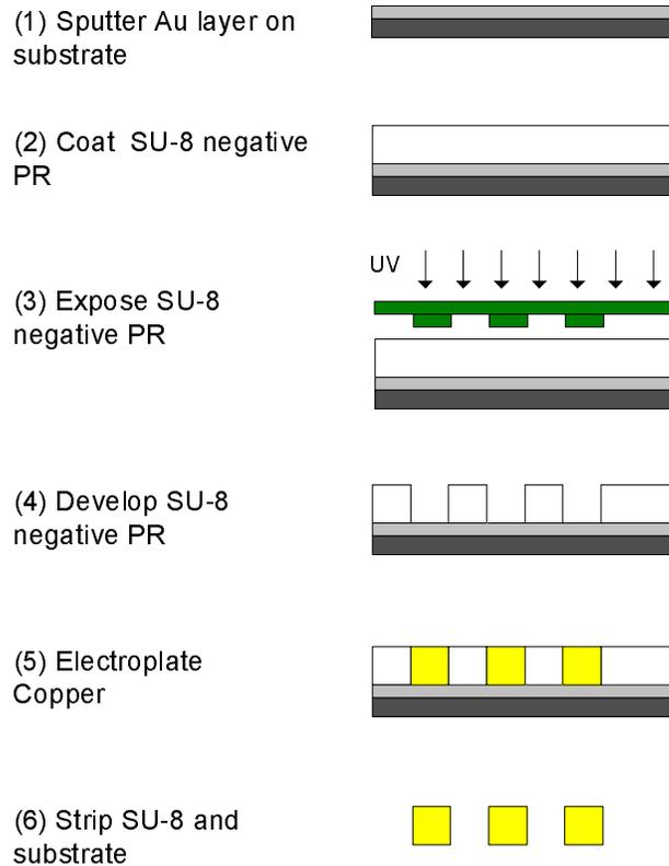
Figure 3.3: Copper spring fabrication process. Photo courtesy of Johnny M. H. Lee
