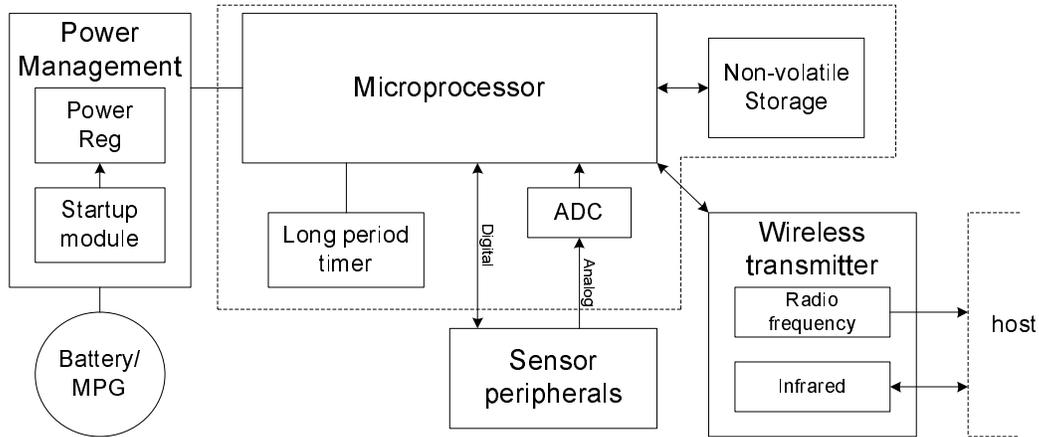
Figure 4.1: Generic platform block diagram
