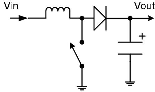
Figure 4.6: Simple boost converter [33]
