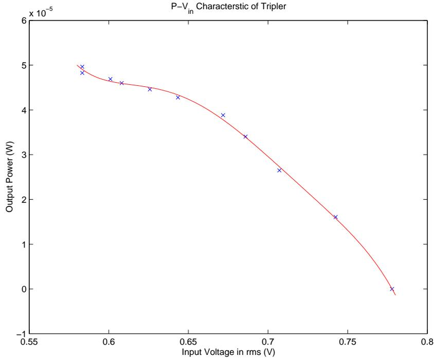
Figure 3.14: Output power versus input voltage of tripler
