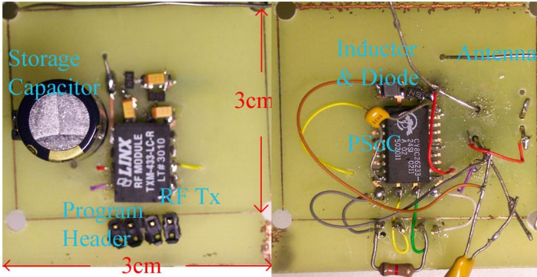
Figure 5.3: Photograph of prototype 2
