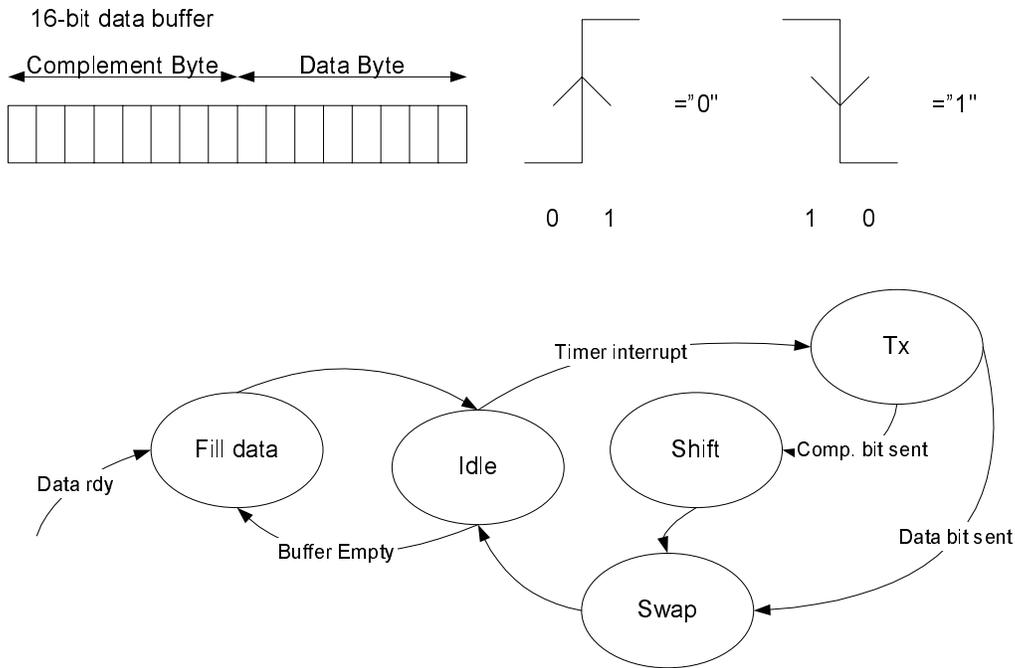
Figure 6.6: State diagram explains Manchester encoding
