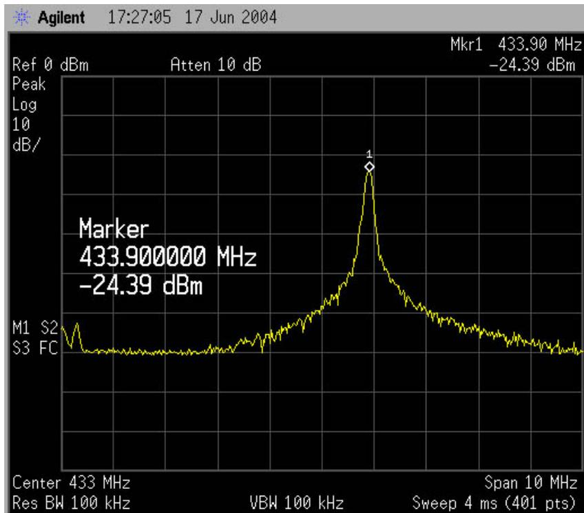
Figure 6.13: Transmission power of the 2D ring at 1 *cm*
