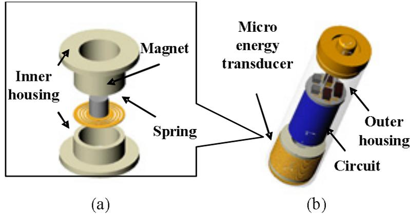
Figure 3.1: Illustrations of: (a) Inner structure of the micro power generator; (b) the AA-size micro power generator which is integrated with a power-management circuit. Photo courtesy of Johnny M. H. Lee
